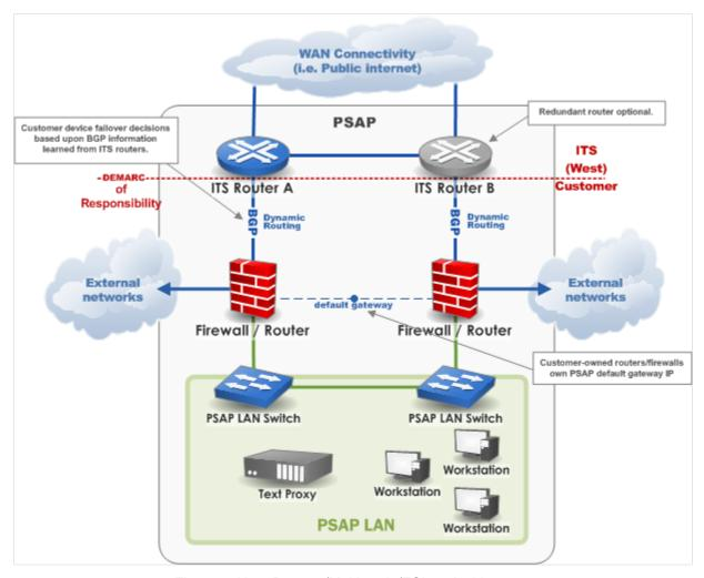
Figure 2: Host-Remote/Multi-node/ESInet Architecture
