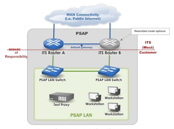
Figure 4: Standalone Isolated PSAP ITS Architecture
