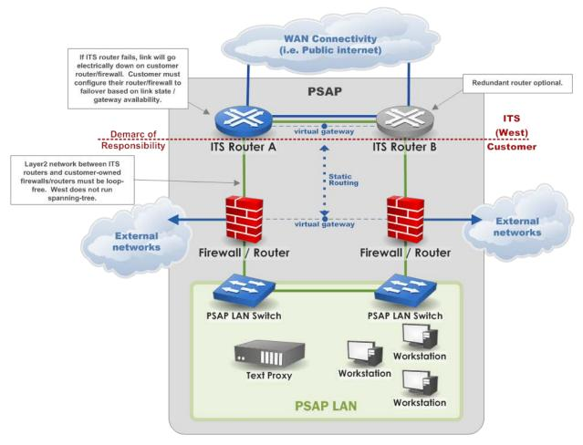
Figure 3: Standalone non-Isolated PSAP ITS Architecture
